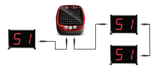
Connect the stereo 3.5mm jack to jack lead supplied, to either of the external display sockets on the RD100, and to either of the external display sockets on the compatible bingo machine.
